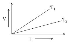
V-I graph for a metallic wire at two different temperatures  $T_1$  and  $T_2$  is as shown in the figure. Which of the two temperatures is higher and why?
