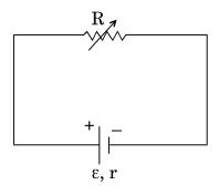
A variable resistor R is connected across a cell of emf  $\epsilon$  and internal resistance r as shown in the figure. Draw a plot showing the variation of (i) terminal voltage V and (ii) the current I, as a function of R.
